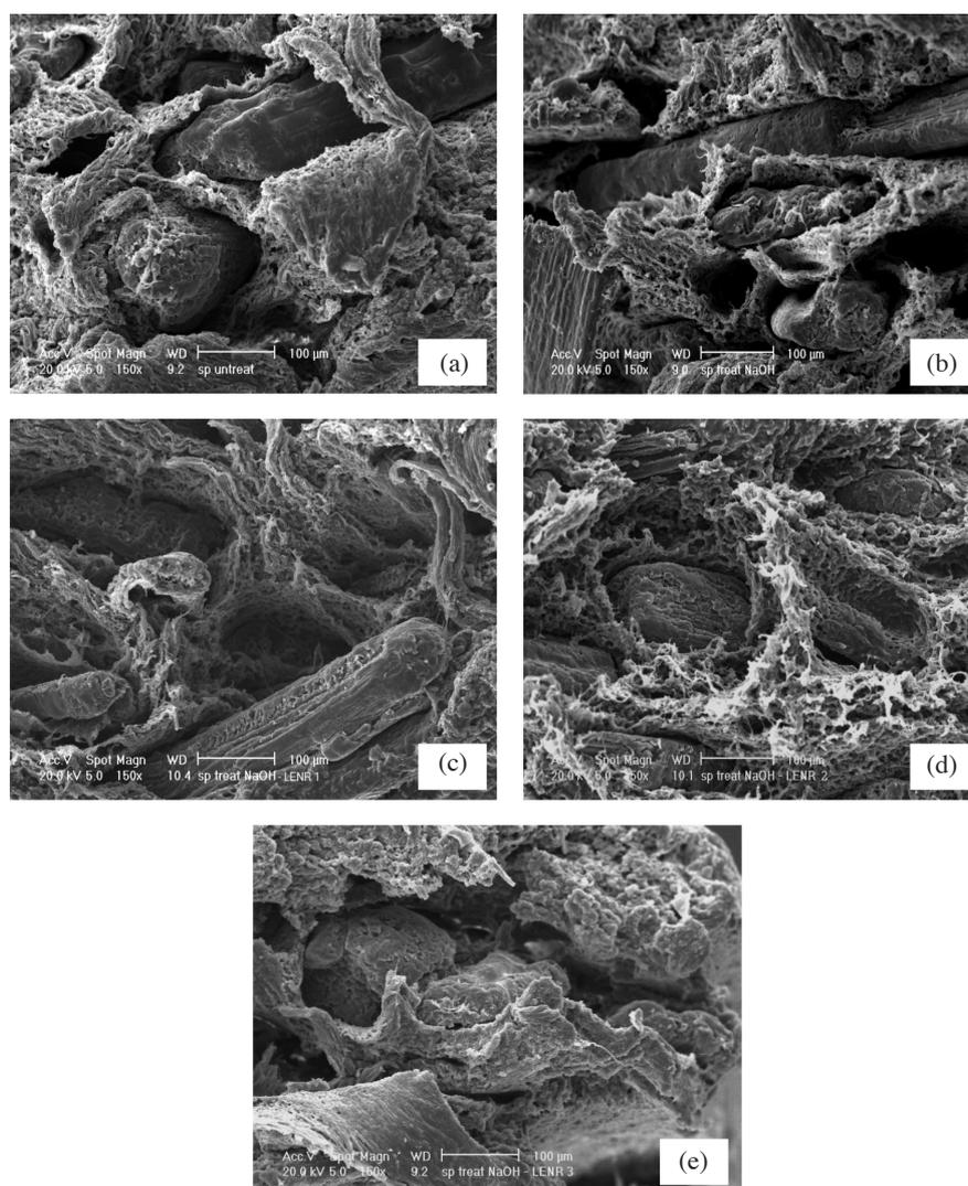
FIGURE 6. SEM micrographs of composites with magnification 150x: (a) TPNR/RHi, (b) TPNR/RHiNa, (c) TPNR/RHiNaLE 1, (d) TPNR/RHiNaLE 2 and (e) TPNR/RHiNaLE 3
