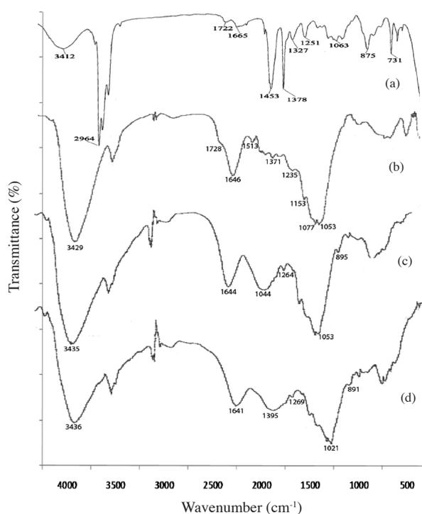
FIGURE 1. FTIR spectra of : (a) LENR, (b) RHi, (c) RHiNa, and (d) RH treated with 5% NaOH-10% LENR (RHiNaLE 2)
